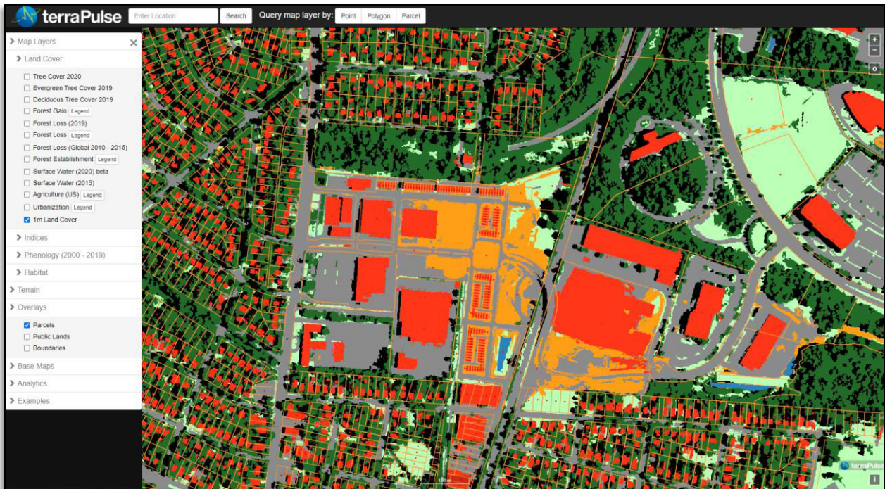
Figure 4. The terraView dashboard showing the 1-meter resolution terraPulse Land Cover Type map over College Park, Maryland. The dataset has six categories: building (red), pavement (gray), tree (dark green), grass/herb (light green), water (blue), and bare (orange). Property parcels are outlined in orange. Note the large patches of bare soil detected during commercial development of large site in the center of the map.
